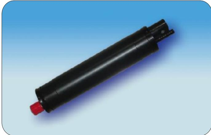
The MONITOR CTD has been developed from Valeport's MIDAS CTD, utilising the same accurate, robust sensors and synchronised sampling technique, but packaged as a smaller, lightweight unit to suit small boat or shallow water applications.
