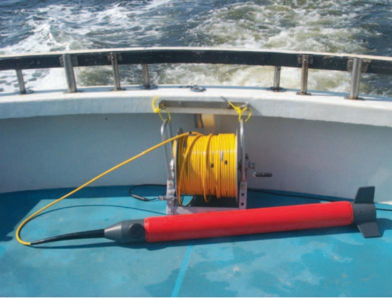
SeaSPY towfish with altimeter and 200m of cable on a metal reel
